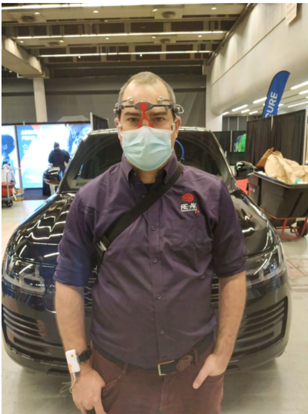
Figure 1: Frédéric Simard, President of Technologies RE-AK wearing the Nucleus-Hermès. The headset measures brain waves and facial muscle activity, while the bracelet measures electrodermal activity and heart dynamics.
